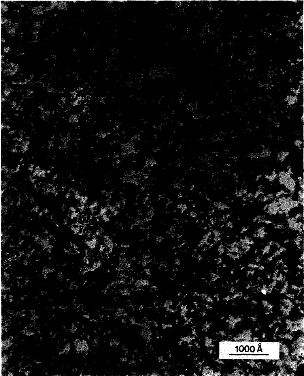
FIG. 2. Typical thin region of freshly reduced Pt/Al 2 O 3 specimen.
